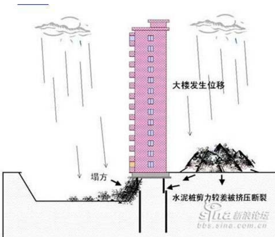
The building began to shift and the concrete pilings were snapped due to the uneven lateral pressures.
